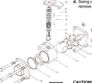
**CAUTION!** Ball and ball seal are sensible to mechanical damage, the surfaces shall not be in contact with any tools.
