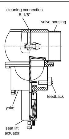
The vacuum valve DELTA VRAH 11 is used in applications in which equipment can be damaged by a vacuum (e.g. in containers or pipelines).
