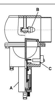
Through the cleaning nozzle **(B)** in the housing, the product-wetted parts of the valve can be cleaned during the cleaning process. Moreover, the contact surfaces between the seat seal and the seat can be cleaned through seat lifting. For this purpose, the seat lift actuator **(A)** is controlled in short intervals during the cleaning process.
