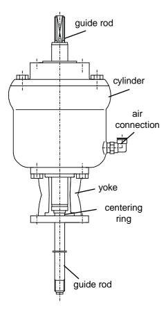
A pneumatic stroke limitation can be used for the valve series DELTA SW4 / M4.
