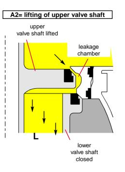
Seat Lift Actuator for Double Seat Valves DELTA D2 / DFplus2 Operating Manual : Rev. 2
